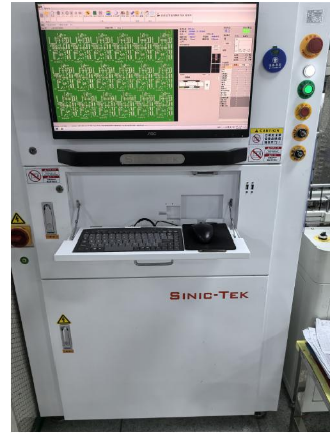
Online solder paste inspection instrument SPI
