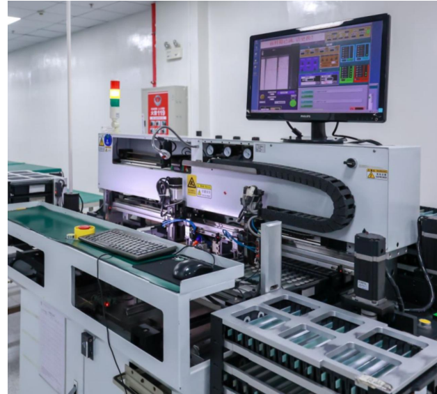
Fully automatic board splitting/testing/sleeving machine : 10 sets
