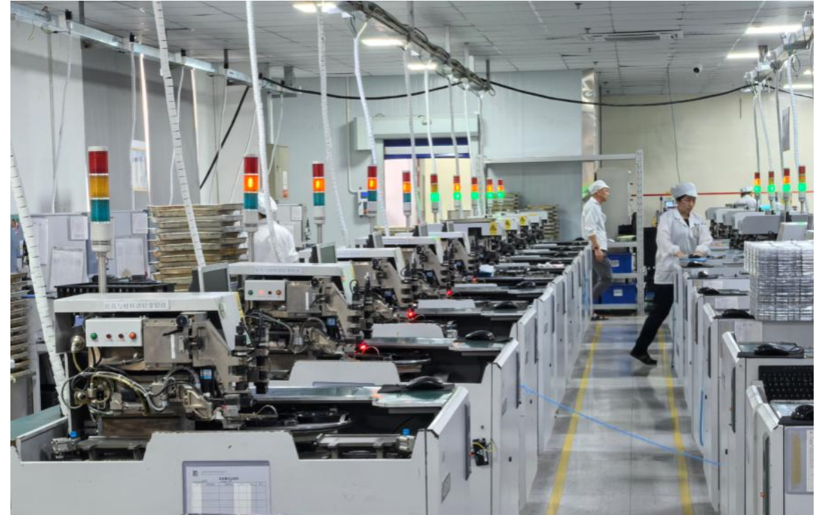
Wire bonding machine: 20 sets
