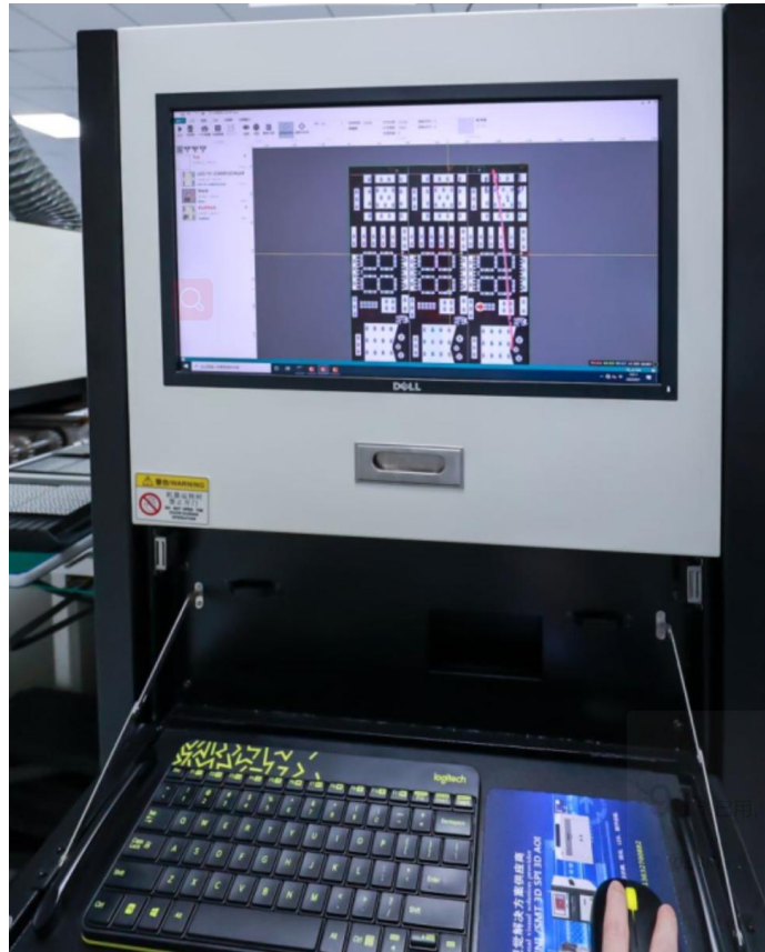
Online AOI tester for PCBA semi-finished products
